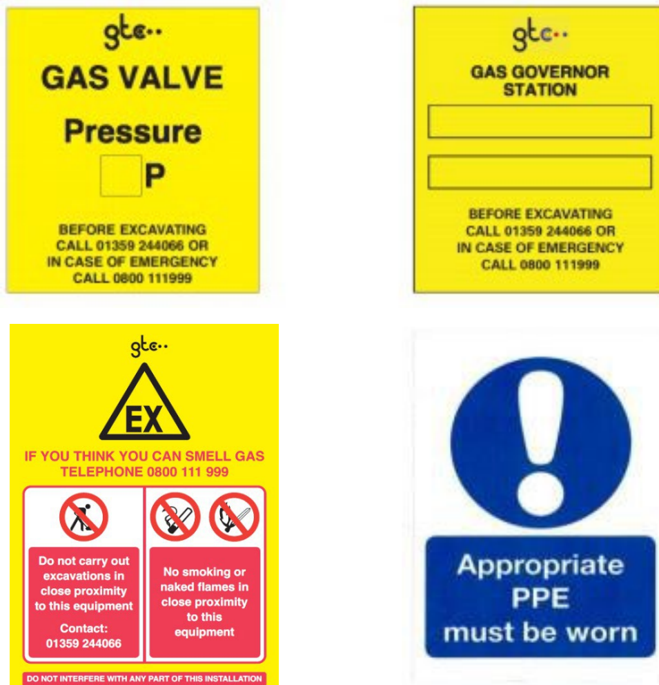
Figure 35. Examples of the signage required
