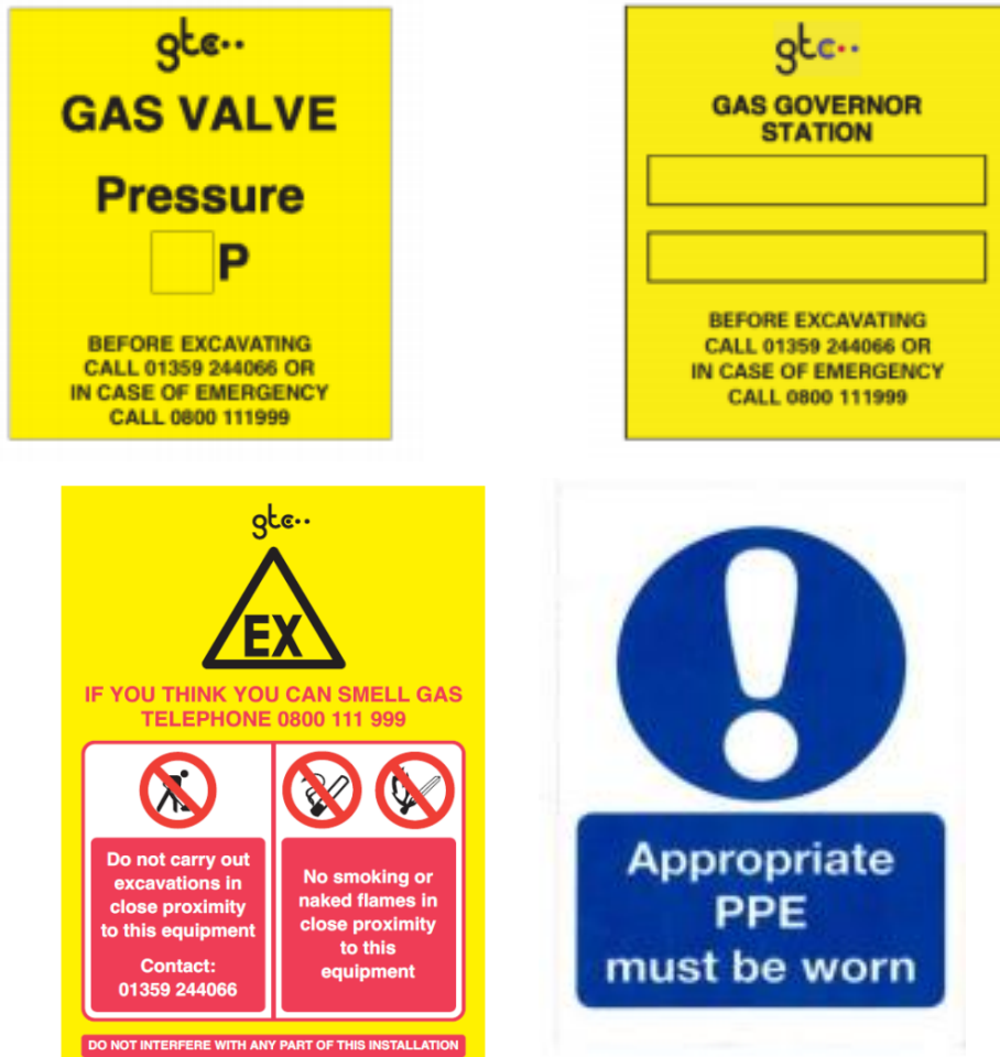
Figure 35 – Examples of the signage required
