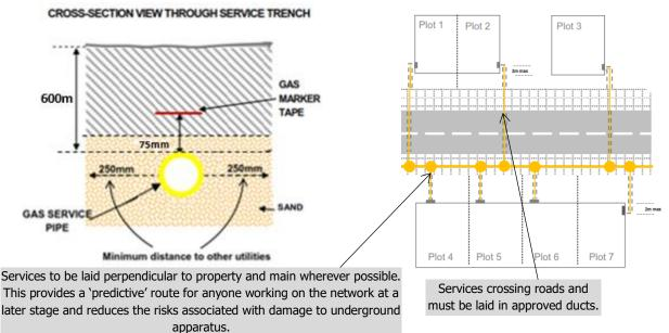
**NOTE**: Services which **CANNOT** follow the designed route due to physical obstructions (e.g. drain covers etc) **MUST** be INDIVIDUALLY agreed with GTC before being laid and the Developer **MUST** produce an as laid drawing showing the agreed route and submit this to GTC prior to the service being connected.
