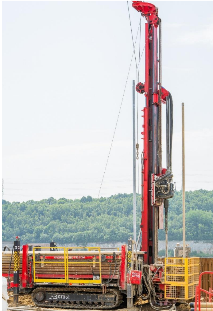
Figure 7: Example of typical rig used for drilling
