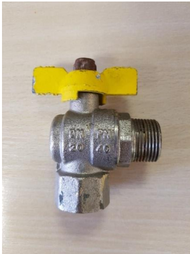
3/4" Female BSP Taper x 3/4" male BSP Taper Angled butterfly valve. No Adaptors available. Valve requires to be replaced.
