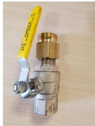
**3/4" female BSP Taper x 3/4" male BSP Taper Valve with 3/4" female BSP Taper x 3/4" BS746 adaptor fitted. (Same adaptor can be used for angled valves with 3/4" male BSP outlet thread).**
