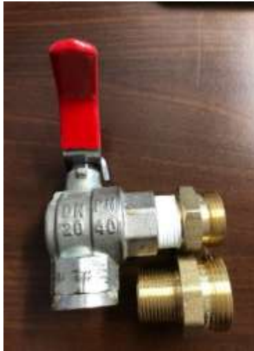
3/4 " Female BSP Taper x 3/4 " Female BSP Taper Angled butterfly Valve with 3/4" BSP x 3/4" or 1" BS746 adaptor and replacement lever handle.
